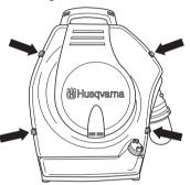
Loosen the two fasteners holding the air filter cowling and remove the filter. Wash the filter clean in warm, soapy water.
